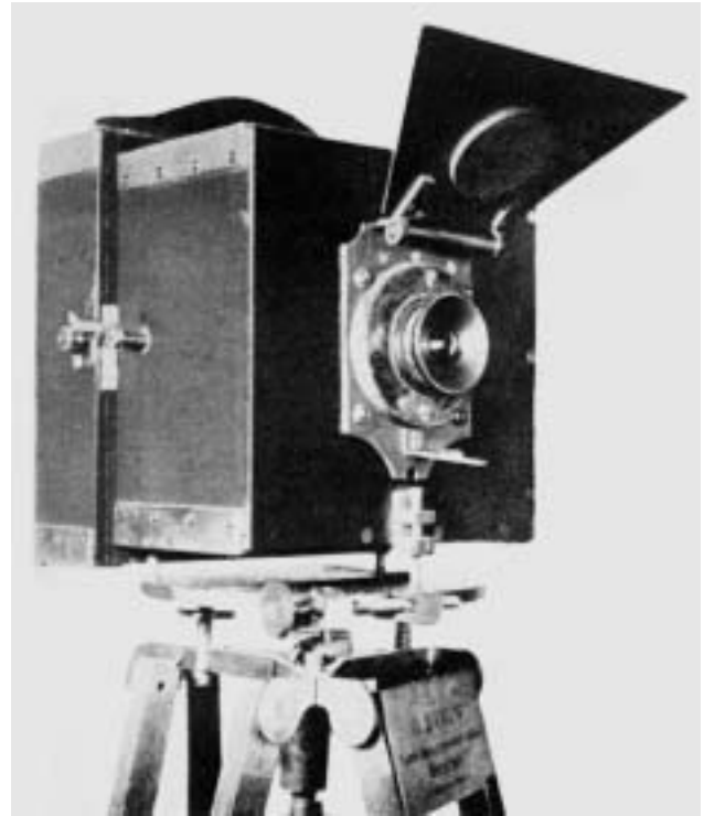
Fig. 3: The first one of Meydenbauers's photogrammetric cameras (built in 1867)
